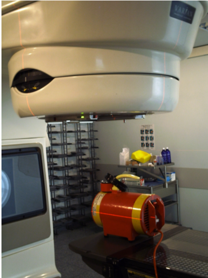
Figure 4.7: Filter paper and vacuum pump device setup in the linear accelerator “Clinac 2100C”.
